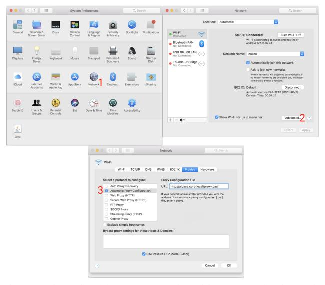
If "Auto Proxy Discovery" is enabled, then Web Proxy Auto-Discovery is in use (see next section). If "Automatic Proxy Configuration" is enabled, the address field contains the PAC URL.
