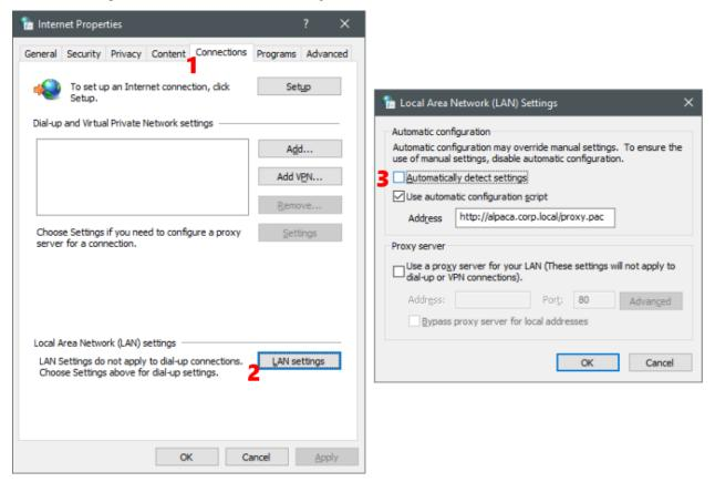
If "automatically detect settings" is enabled, then Web Proxy Auto-Discovery is in use (see next section). If "use automatic configuration script" is enabled, the address field contains the PAC URL.
